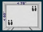
In an elevator with minimum dimensions of less than 60 x 78 inches, two people can stand in opposing corners.
